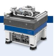
The standard XYZT planar platform includes an ETEL ZT combined module on the gantry beam of the XY stage. The ZT combined module provides infinite Theta rotation and dual Z-axes: a coarse Z axis for wafer loading and unloading, and a fine Z axis for fine adjustment.
